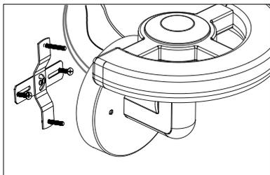
2. Pull the power supply wires to the side and install the fixture crossbar onto the J-box with the screws provided (Fig B).
