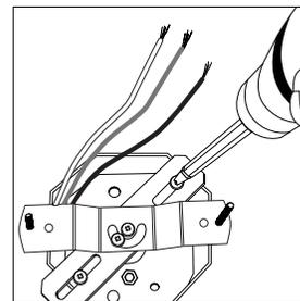
3. Using the wire nuts provided, connect the bare grounding wires from the fixture to the house ground. Connect the white fixture wire to the neutral house wire. Connect the black fixture wire to the power supply wire (Fig C).
