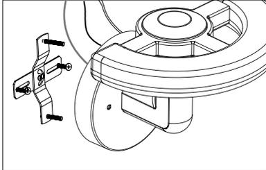
2. Before installing the round plate, add silicone sealant between the rear of the round plate and the J-box. Pull the power supply wires through the round plate and install the round plate along with crossbar, onto the J -box with the screws provided (Fig B).
