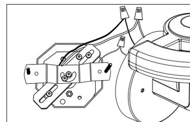
5. Position into place and secure fixture by installing the rubber washers and the canopy mounting nuts, then tighten the nuts (Fig E).
