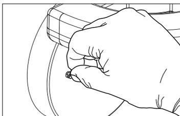
6. Caulk between the light fixture and the wall surface with a silicone sealant (not included).
