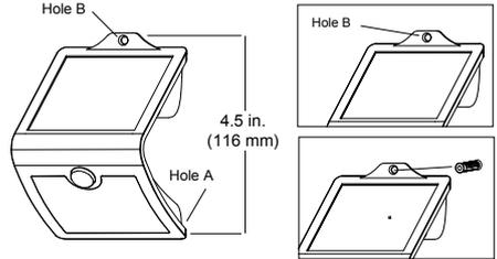
3. Align the top of fixture to the hole created and insert a screw (provided) into hole B and tighten (Fig. C).
