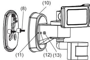
7. Once the fixture is tightly secured to the j-box, apply a silicone sealant around the base of the fixture to prevent moisture from reaching the connections.
