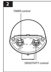
Once the fixture has been tested for proper Sensitivity, rotate the TIMER rotary control knob into the Timer settings. The timer settings indicate how long the light stays on after the PIR senses motion at night only.
