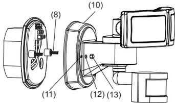
7. Once the fixture is tightly secured to the j-box, apply a silicone sealant around the base of the fixture to prevent moisture from reaching the connections.
