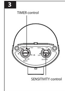
If Dusk to Dawn is desired, rotate the TIMER rotary control knob to the "D2D" position, the light turns on at dusk and off at dawn automatically, regardless of the presence of motion. The "D2D" setting ensures lights are non-operational in daylight and only function at night.
