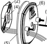
5. Connect the power supply wires directly to the terminal block (7). Secure the wires to the terminal block by using a small screwdriver.
